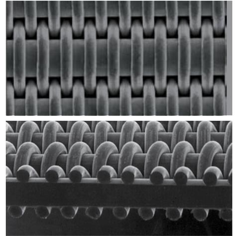
RPD – Reverse Plain Dutch Weave. Like the MINIMESH® SPW-S, the MINIMESH® RPD-S is a plain weave filter mesh, but features a reverse wire diameter arrangement. The MINIMESH® RPD-S consists of thin warp wires positioned close to each other and thicker weft wire, woven in at a defined distance. The resulting strength in the warp direction makes the MINIMESH® RPD-S a popular choice as a filter belt. Moreover, the versatile, reverse plain Dutch weave is used in applications
