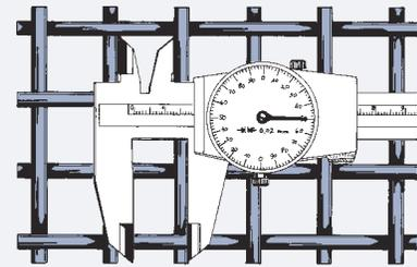
Vernier caliper for measuring aperture widths of more than 4mm. It can also be used for aperture widths of greater than 10mm.
