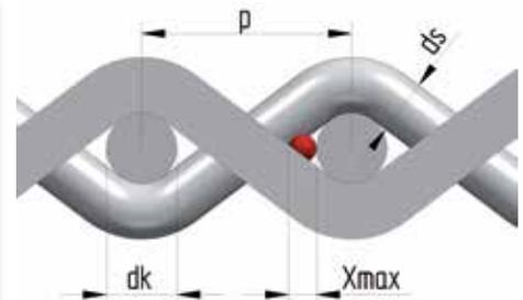
The heart of the MINIMESH® S filter generation: Precision pores with precisely defined geometry.
