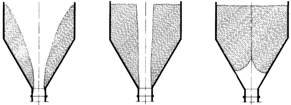
By installing PLYMESH aeration pads it is possible to avoid problems, such as funnelling, ratholing and bridging formation.
