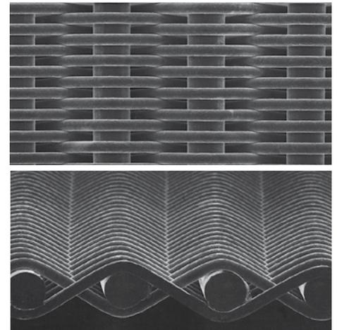
The MINIMESH® HIFLO-S filter weave corresponds to the pore size range of MINIMESH® SPW-S. In utilizing ultra-fine wires woven in a plain weave, a larger number of pores per unit area is achieved, allowing a high throughput rate despite the small pore size. The MINIMESH® HIFLO-S is a surface filter, meaning the smallest pore is determined by the distance between weft wires and not by the pores within the three-dimensional filter weave. Cleaning, back flushing, and strength
