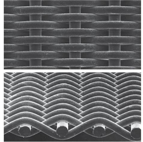
SPW – Single Plain Dutch Weave. Weft wires are woven in a plain weave without space between them, making the aperture width zero. Because there is approximately five times more weft wires than warp wires, the strength is higher in the weft direction. The SPW filter weave is used for surface filtration and noted for its ease of cleaning and back flushing. The pore size of the most common MINIMESH® SPW filter is within the range of 40µm to 300µm. To reduce
