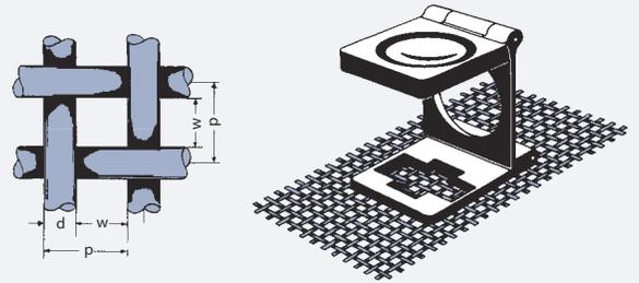
Counting glass for measuring aperture widths less than 1mm in a row with determined length.
