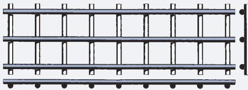
Pressure Welded Screen, Type F
