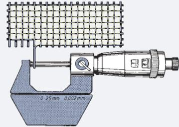
Micrometer screw used to determine wire diameter.
