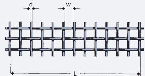
Measuring row with determined length for aperture widths of 1mm to 16mm.
