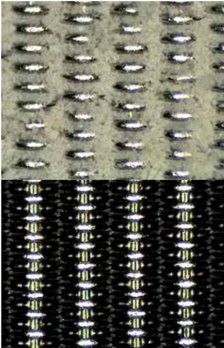
Dirt holding capacity of a HIFLO 30-S.
