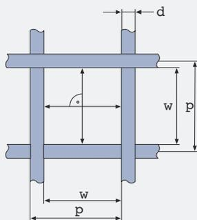
The number of apertures per unit length ( $n$ ) is the number of apertures counted in a row one behind the other for a given unit length. The unit length may be 1cm, 1dm, 1in, or any other unit of length; however, the number of apertures with a length of 25.4mm is designated as "Mesh".
