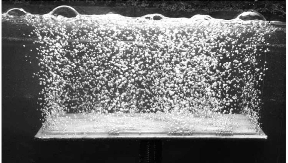
Uniform penetration of air through the PLYMESH aeration pad demonstrated in a water bath.
