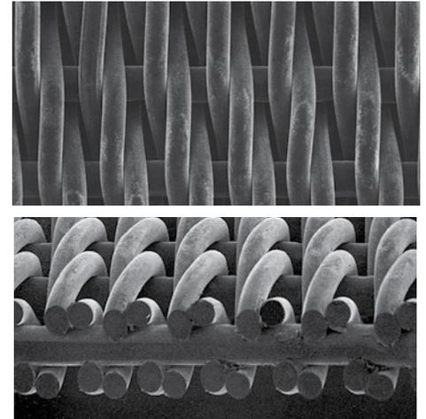
MINIMESH® TRD-S is comparable to the reverse plain Dutch weave; however, the warp wire is woven in a 2/2 twilled weave, giving it the advantage of lesser distortion for the warp wires. The resulting strength in the warp direction favors applications like a filtration belt.
