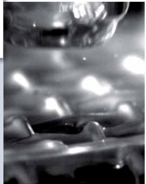
As an additional quality assurance measure, MINIMESH® S metal filter cloths are bubble point tested. According to the customer's wishes, the determination and specification of filter characteristics is performed using first bubble, mean pore size, or both of these parameters.
