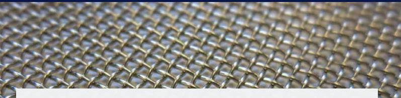
Aperture width (labeled w in the below diagram) is the distance between two adjacent warp or weft wires, measured in the projected plane at the mid positions.
